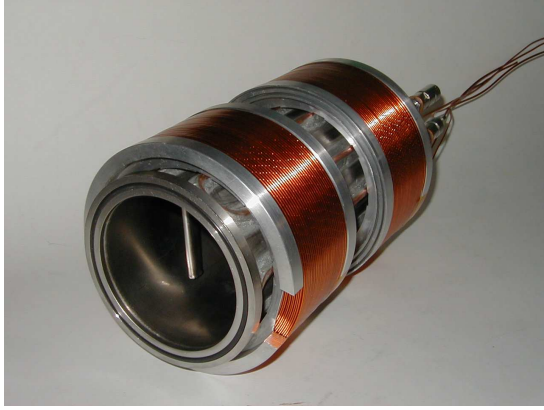
Figure 13: The source body with the new solenoids.
