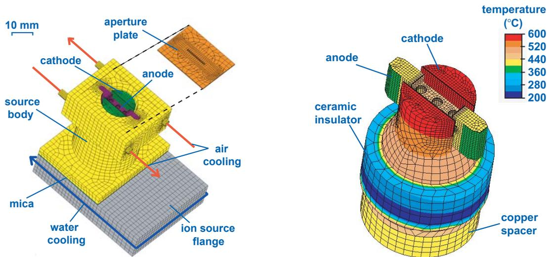
Figure 3: ALGOR thermal model of the ISIS ion source. Figure 4: Component temperatures from the steady state model.
