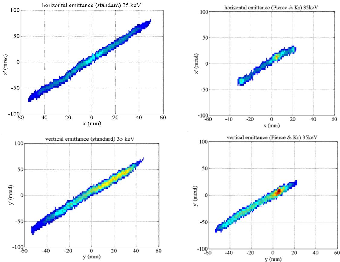
**Figure 9:** ISDR horizontal and vertical emittance plots for the ISIS standard geometry and old pole pieces with no introduction of Kr.
