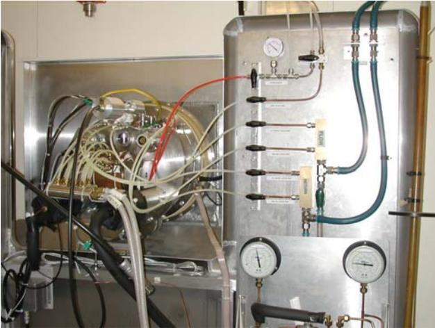
**Figure 1:** The top loading ion source mounting flange.
