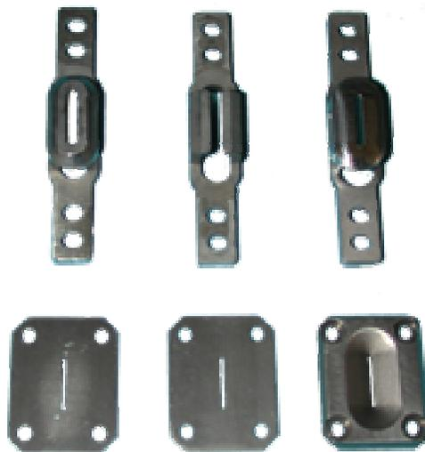
**Figure 8:** Extraction electrodes and aperture plates for the ISIS standard geometry (centre), terminated standard geometry (left) and Pierce geometry (right).
