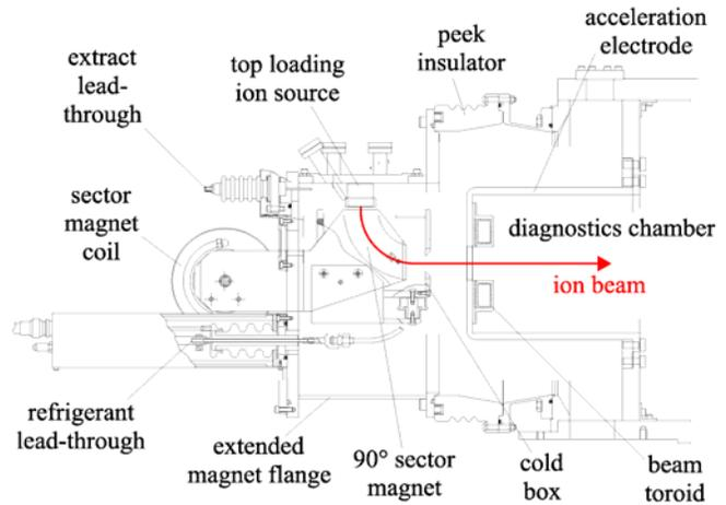
**Figure 2:** Schematic of the top loading ion source.
