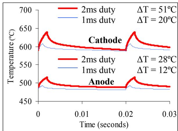
**Figure 7:** Anode and cathode surface temperatures for 1 ms and 2 ms duty cycles for the double sized ion source calculated from the transient model.
