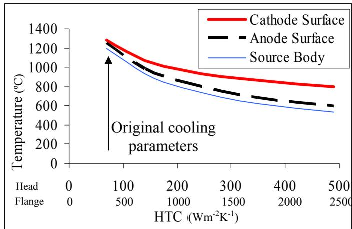
**Figure 5:** 1 ms duty source steady state temperatures for increased cooling.
