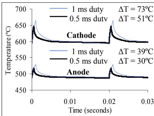
**Figure 6:** Anode and cathode surface temperatures for 0.5 ms and 1 ms duty cycles for the normal sized ion source calculated from the transient model.
