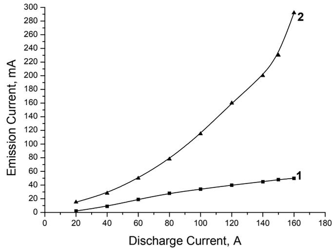
Figure 2. Dependence of negative ions current (curve 1) and accompanying electrons current (curve 2) on discharge current.
