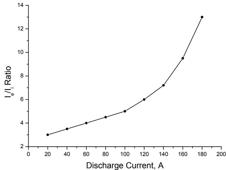
Figure 5. Dependence of  $I_e/I_i$  ratio as a function of discharge current.
