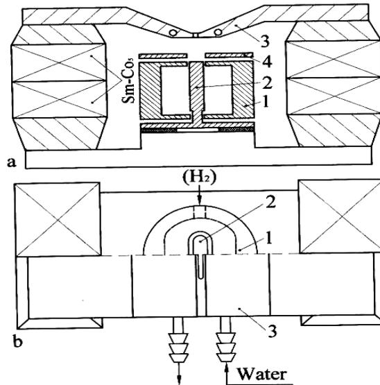
Figure 3. Ion source with slot-hole geometry.
