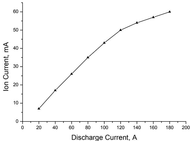
Figure 4. Dependence of  $H^-$  ion current on the discharge current.
